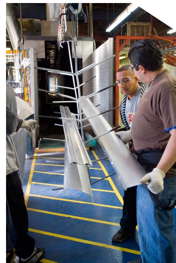
Extruded aluminum parts in prep for powder coating.
